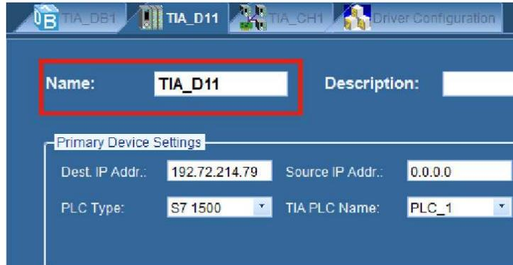
Picture 22: Device name is part of the I/O address
